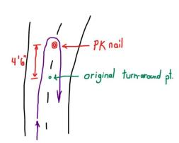
This illustration shows how I modified the initial course to ensure the proper adjustment was applied to get 5,000m. after seeing that the calculations were 9' 0" short of 5,000m.
